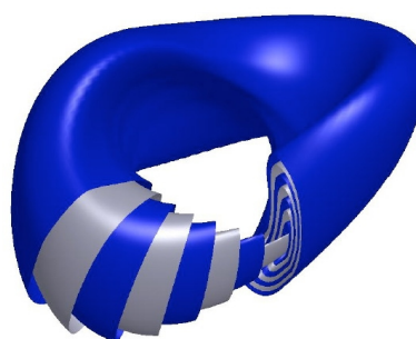
The nested magnetic surfaces of the Columbia Non-neutral Torus
